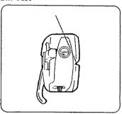
Place bobbin in bobbin case Pull thread through slot of case
